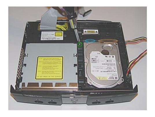
With the hard disk removed you must now remove two torx 10 screws as indicated by the yellow circles.
