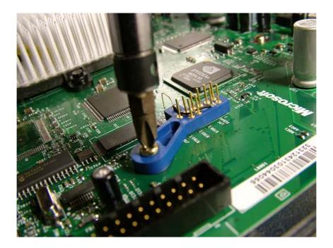
Ensure that the d0 wire is firmly in position once the screw has been tightened.
