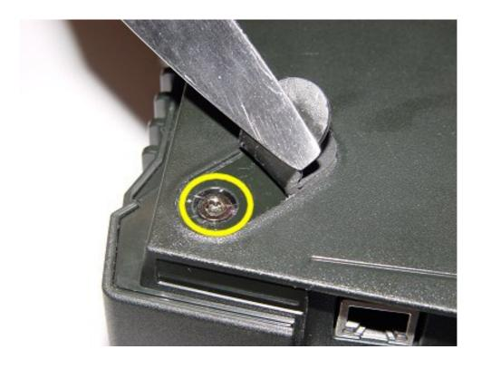
Firmly remove the console's cover and you will reveal the contents of the Xbox!
