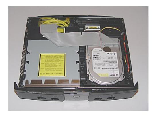
Now remove the IDE cable (marked in orange) and the power cable (blue) from the hard disk drive.
