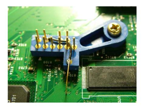
Position the Xenium on the solderless adaptor as shown in the photo below, ensure that both rows of pins on the adaptor are correctly lined up to the Xenium's pin header and gently push the Xenium into position.
