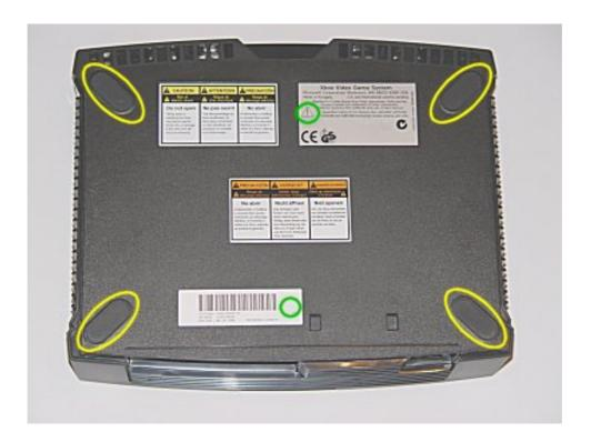
You will need to lift the consoles feet up as displayed in the picture below to access four of the torx screws. The green circles above indicate the location of two torx screws that are hidden under stickers, remember that breaking these stickers will void your warranty but it is the only way that you can install the Xenium.
