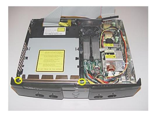
Remove the IDE and power cables from the DVD-Rom drive as indicated by the red and blue circles. You can then remove the DVD-Rom unit and the IDE & Power cables.
