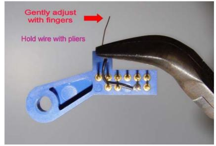
Once you have determined which d0 point you wish to use for your installation, insert the tip of the gold wire into the d0 point and then seat the adaptor over the LPC points. The spring loaded pins of the adaptor should lock into the rivets (or solder) and the adaptor should be positioned as shown below.
